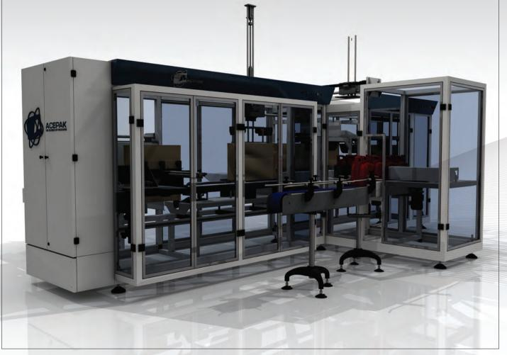
FULLY AUTOMATIC OFFSET INLINE TOP LOADING CASE PACKER. USES REGULAR SLOTTED CARTONS WITH FLAPS OPENING FROM THE TOP. WITH CASE BOTTOM FIRST BEING SEALED AND THEN INDEXED TO THE PRODUCT LOADING STATION WHERE PRODUCT IS PICK AND PLACED, OR DROP PACKED INTO THE CASE. THE CASE IS THEN GLUED SHUT. SUITED TO A WIDE RANGE OF PRODUCT.
