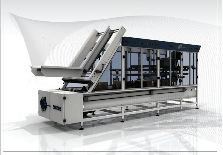
FULLY AUTOMATIC OFFSET INLINE END LOADING CASE PACKER. USES REGULAR SLOTTED CARTONS WITH FLAPS OPENING FROM THE SIDES. WITH INDEXED ACTION CASE FORMING AND LOADING. PRE-COLLATION OF PACKS INTO OPENED CARTONS. VERSATILE AND SUITED TO A LARGE RANGE OF PRODUCTS.
